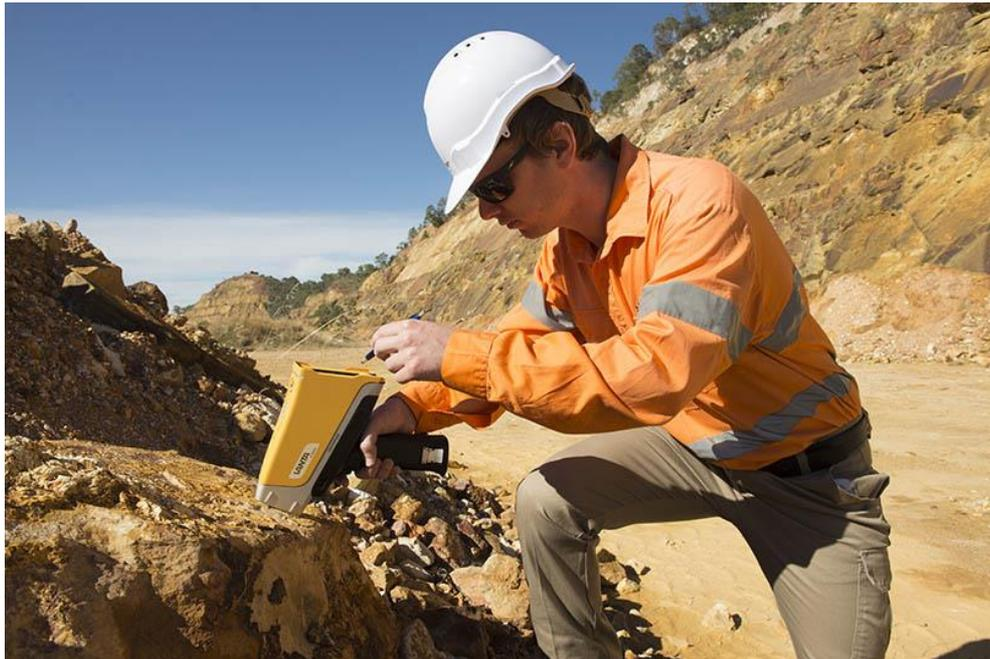
**FIGURE 1: PXR ANALYSIS ALLOWS GEOLOGISTS TO ANALYSE SAMPLE GEOCHEMISTRY IN THE FIELD. (SOURCE: WWW.OLYMPUS-IMS.COM)**
