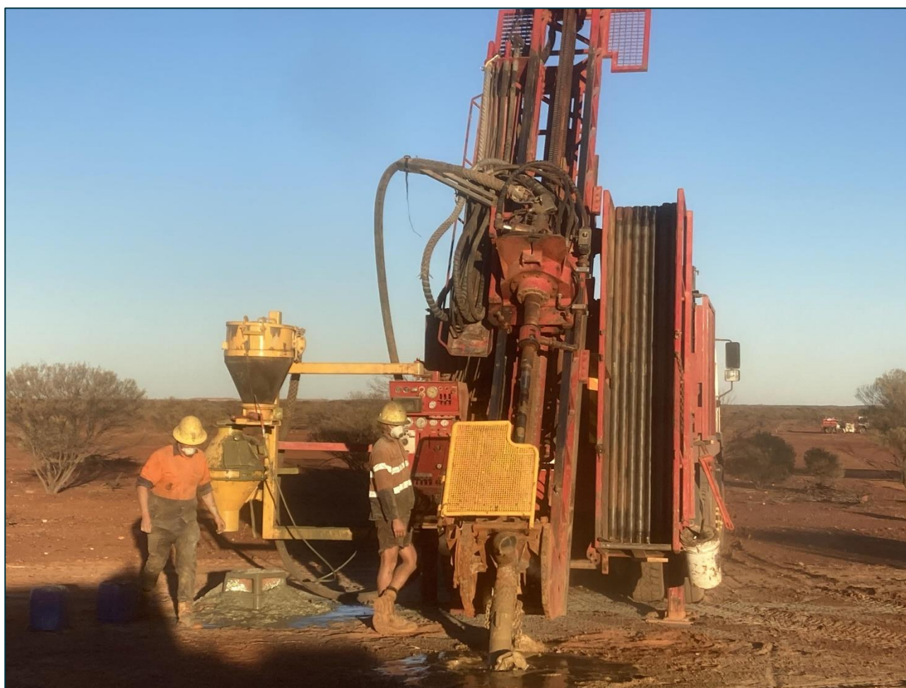
FIGURE 1: AC DRILLING AT SIDE WELL
