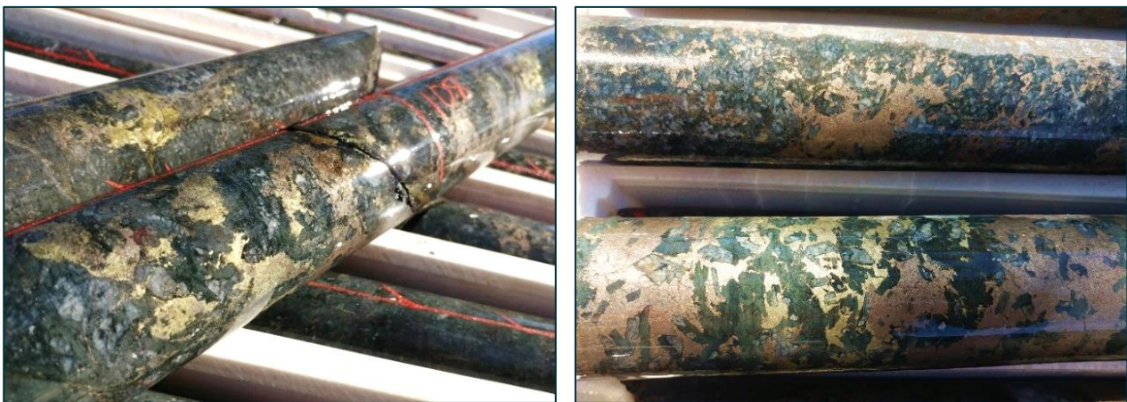
FIGURE 2: CHALCOPYRITE-PYRRHOTITE MINERALISATION IN MT VENN DRILL CORE
