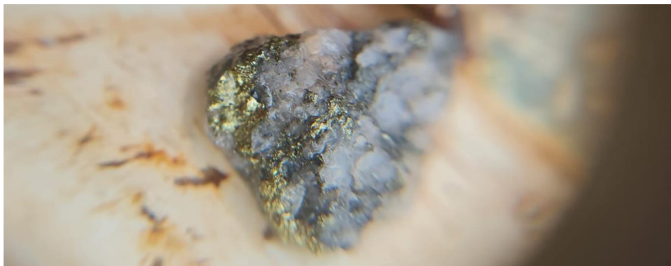
FIGURE 2: A BOTTOM-OF-HOLE CHIP FROM 21MBAC119 SHOWS CHALCOPYRITE-PYRITE MINERALISATION. COPPER ASSAYS ARE NOT YET AVAILABLE.
