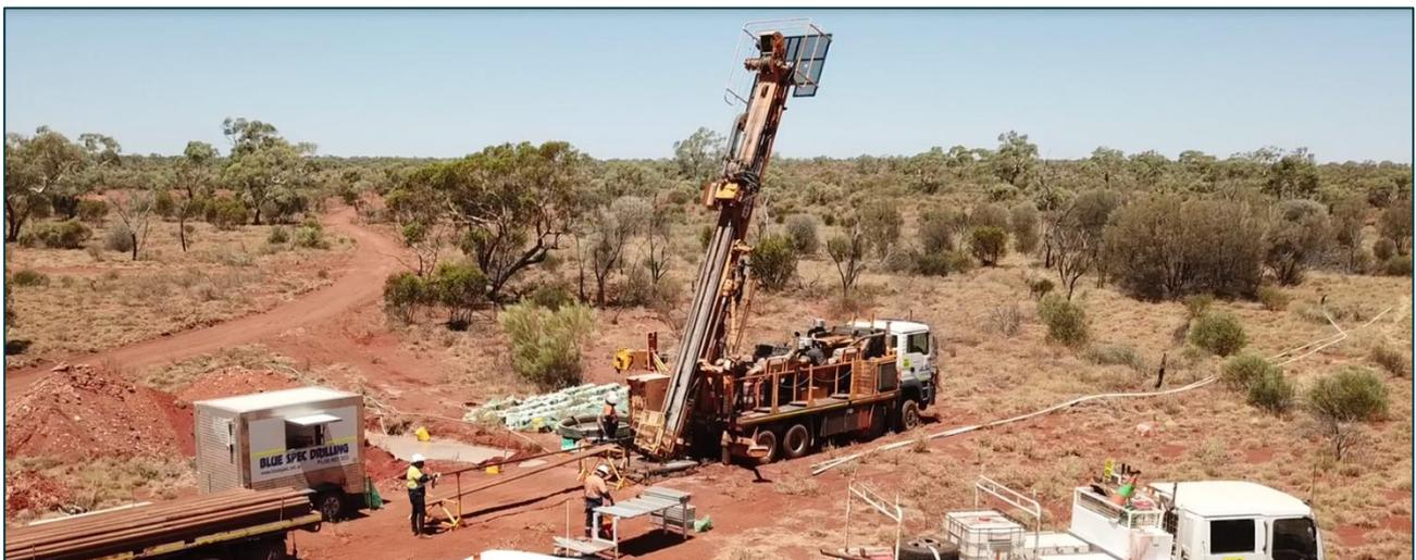
**Figure 3:** Diamond drilling underway at the Zermatt prospect
