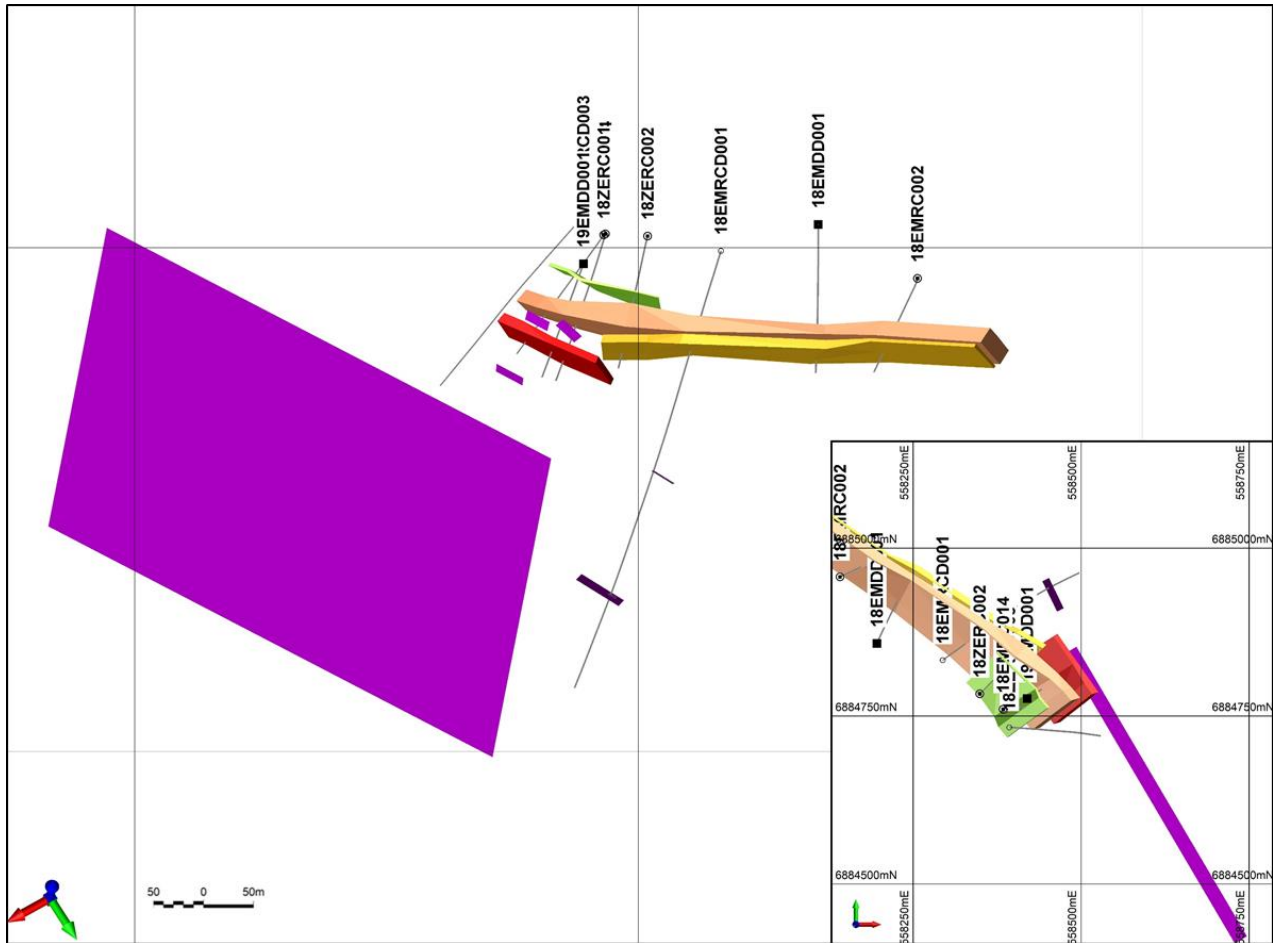
Figure 2. Oblique view of Zermatt modelled sulphide lenses (wireframes) with drilling and new DHEM conductor plates (magenta)
